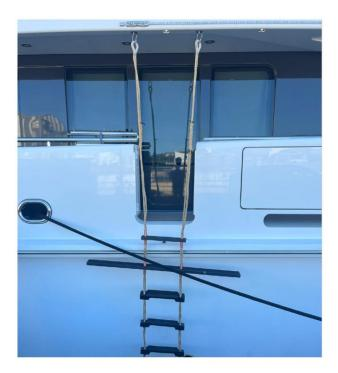
Pilot ladder secured to deckhead (prohibited from 01.01.2028), no vertical handholds, rubbing rail obstruction (albeit relatively minor in this instance)
