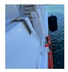
Improper securing of pilot ladders to handrails or fender saddles, no vertical handholds
