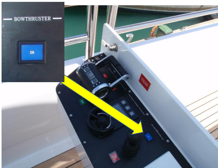
Figure 5: "Blue Light" believed by deckhand to indicate console status
