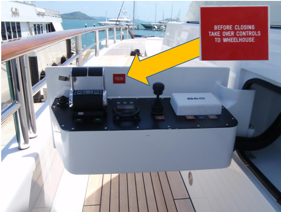
Figure 3 View of plastic warning sign
