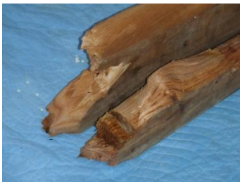
Figure 19: Bollard Walles Failure
