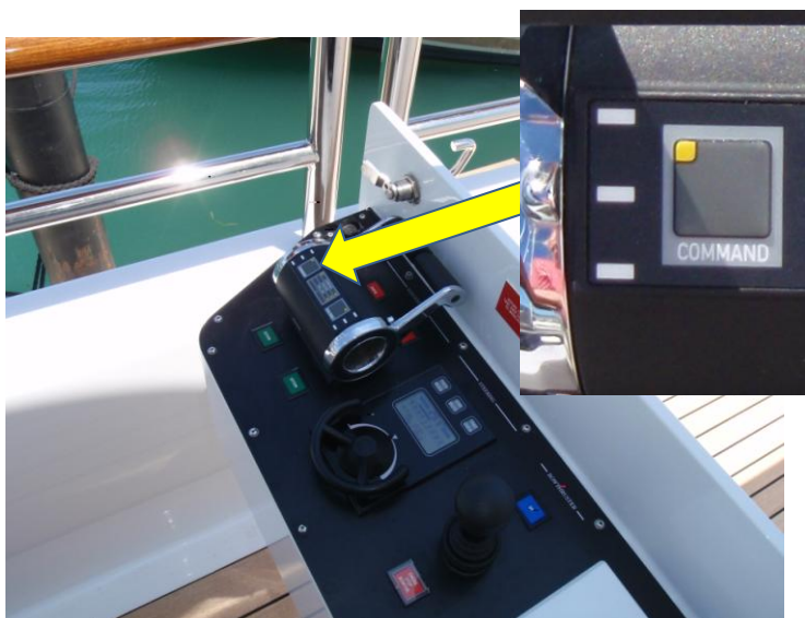
Figure 6: "Yellow Light" indicating Engine Control
