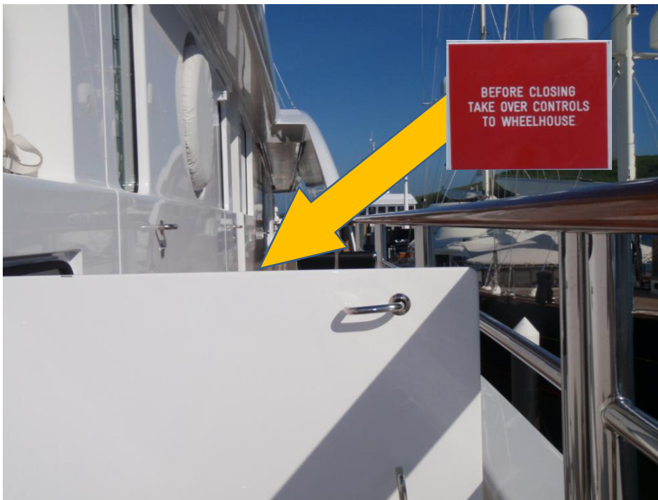
Figure 4: Deckhand's view of console with warning sign obscured
