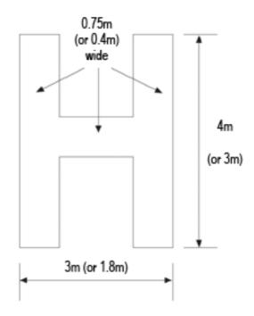
Figure 6 – Dimensions of 'H"
