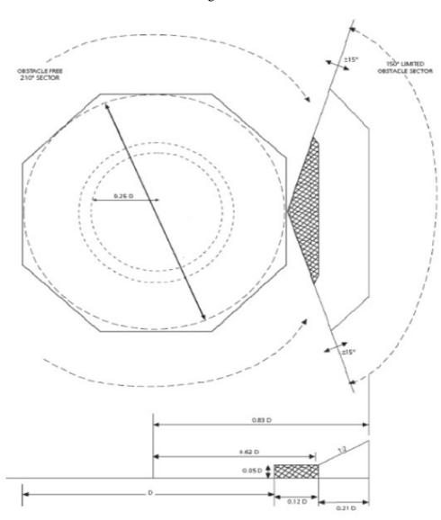
Figure 2 - Obstacle Limitation showing position of Aiming Circle
