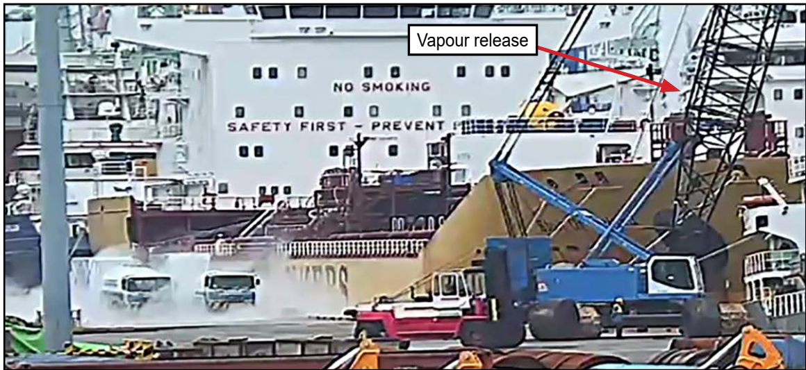
Figure 3: CCTV still showing vapour release from 9S p/v valve
