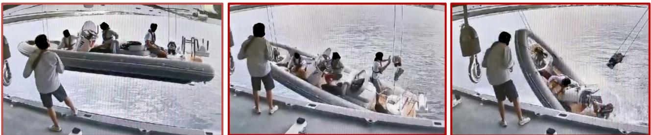
Fortunately, none of the crewmembers on board the tender were seriously injured during the incident. However, serious injuries to the crewmembers could easily have occurred as a result of the fall to the water or by contact with the free-swinging hook and release gear.
