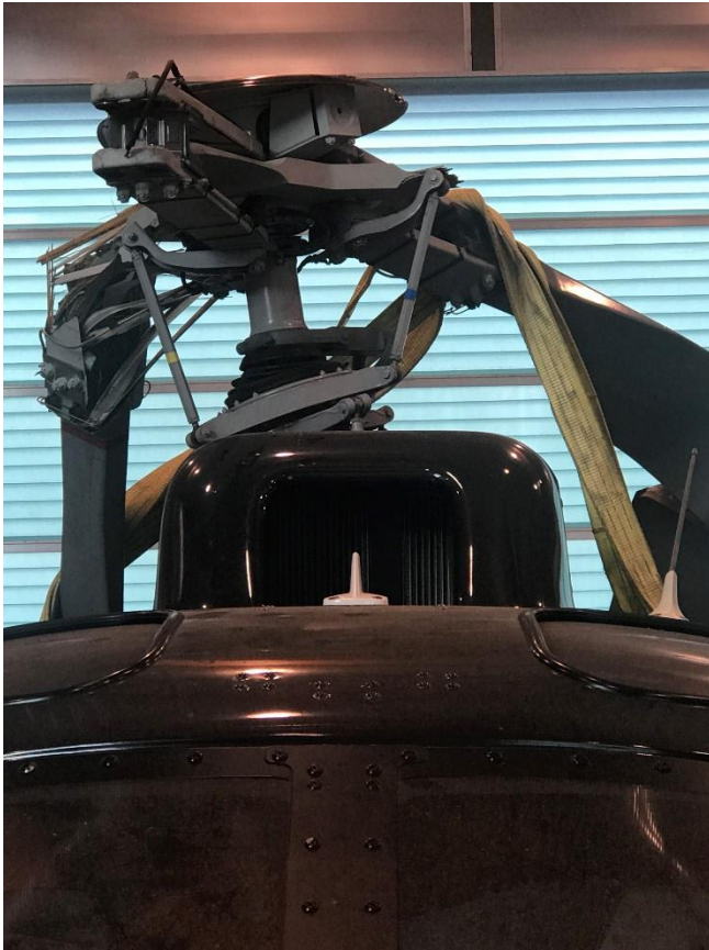
Figure 7: Main gearbox displacement. Photo: AIBN
