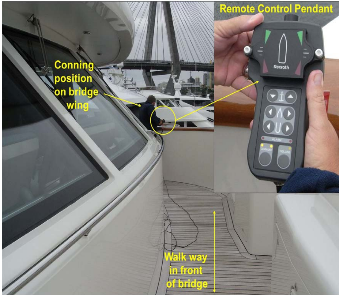
Figure 12: Conning position during manoeuvring
