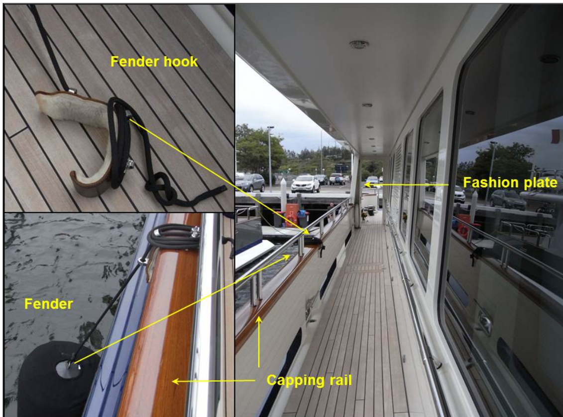
Figure 6: Fender Hook position on capping rail
